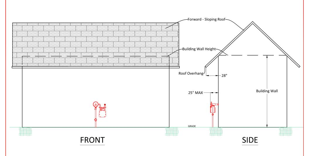
**NOTE 1:** Locate the gas meter on a wall beneath a forward-sloping or hipped roof, where the roofing material is either composite or metal, the overhang is at least 28 inches, and the wall height is less than 25 feet.
