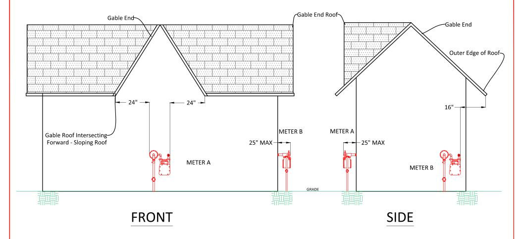
**NOTE 1:** Locate the gas meter on a wall beneath the gable-end of the roof with at least 16 inches from the outer edge of the roof and at least 24 inches from where the gable intersects with a forward-sloping roof. Locate a gas meter on a wall beneath a flat roof only if the overhang is at least 28 inches and the gas meter can be placed at least 16 inches from the outer edge of the roof.
