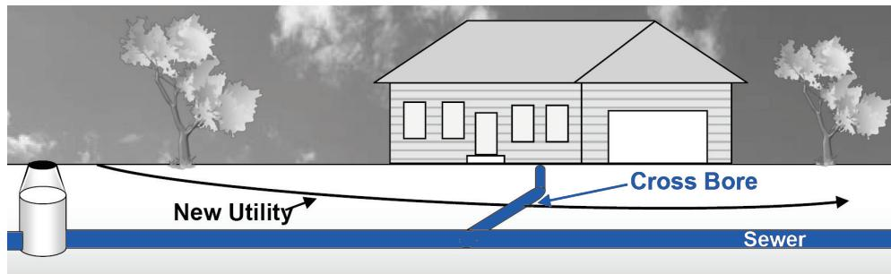
Sometimes the gas pipeline serving a house is accidentally installed so that it crosses through the sewer pipeline. This is called a cross bore, which may occur when trenchless technology is used to install gas pipelines or when sewer lines were not mapped or installed with locatable technology.
